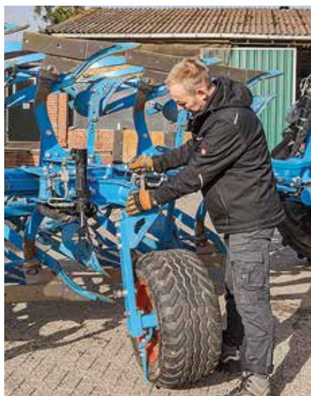
The depth wheel needs to be swapped over for travelling on the road. The transport settings can be conveniently selected on the terminal.
