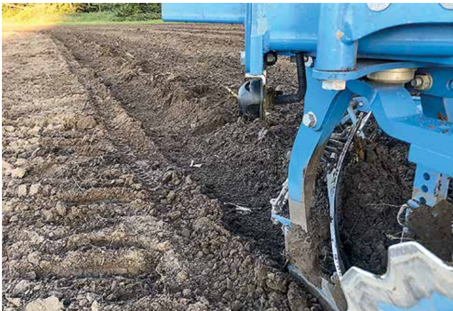
The last furrow: when you need to shallow the back body, the operator just presses a button.
