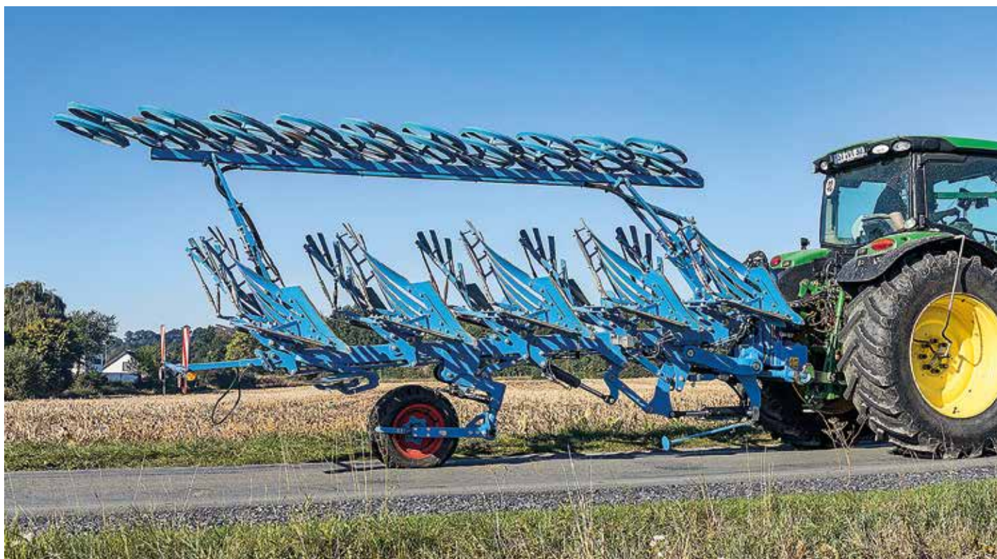
The depth wheel needs to be swapped over for travelling on the road. The transport settings can be conveniently selected on the terminal.
