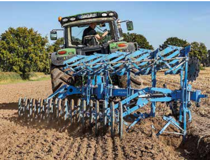
The FlexPack can be raised out of work. The electronics make it possible to quickly change the settings.
